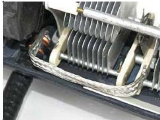
Variable capacitor soldering joints made with RG213 coaxial braid.
