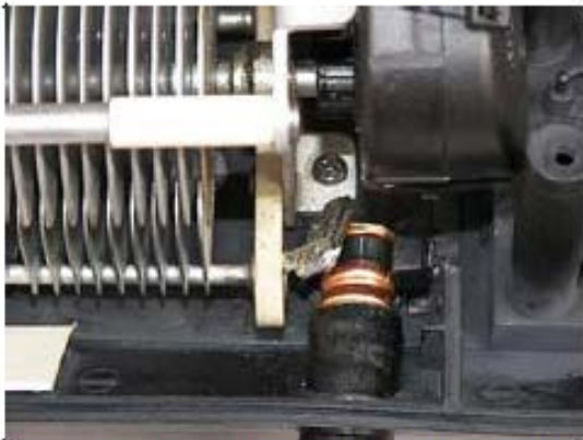
Variable capacitor soldering joints made with RG213 coaxial braid.
