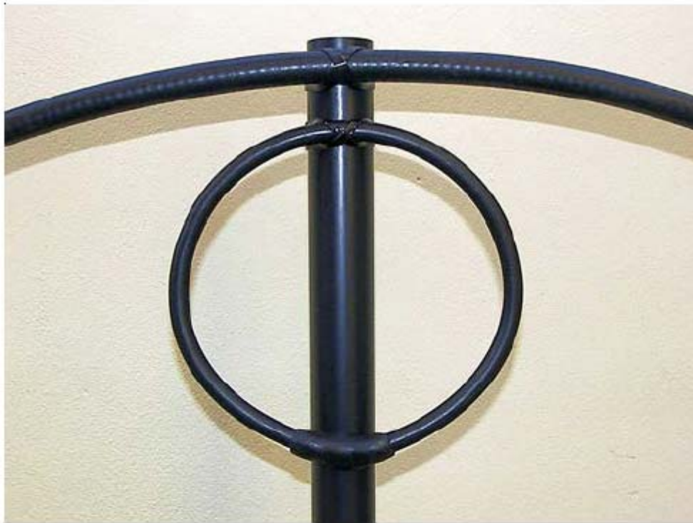
Inner loop made with 56 centimeters of RG213 coaxial cable.
